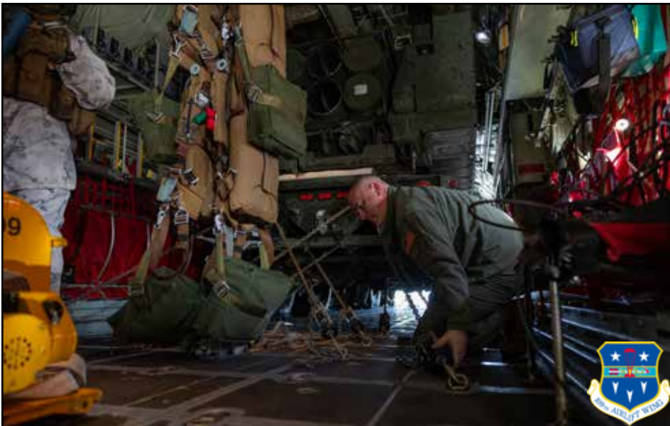
Air National Guard Senior Master Sgt. Dylan Hassis, a loadmaster with the New York Air National Guard 109th Airlift Wing, tightens the tie-down straps securing a High Mobility Artillery Rocket to a C-130 Hercules aircraft in support of Arctic Edge 24 at Eielson Air Force Base, Alaska, Feb. 24, 2024. Photo by Tech. Sgt. Madison Scaringe, 109th Airlift Wing.
