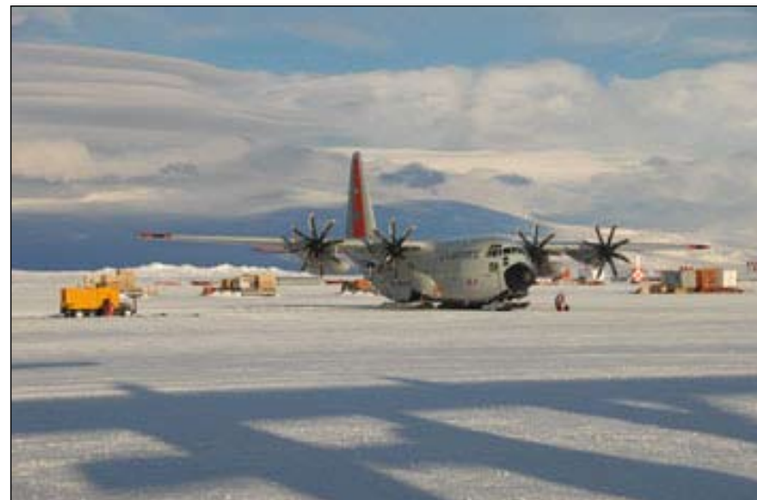
New 8-bladed propellers are being tested on aircraft 92.
