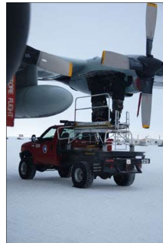
Airmen with the Engine Shop check Magnetic Drain Plugs during a Basic Postflight Inspection after a mission.
