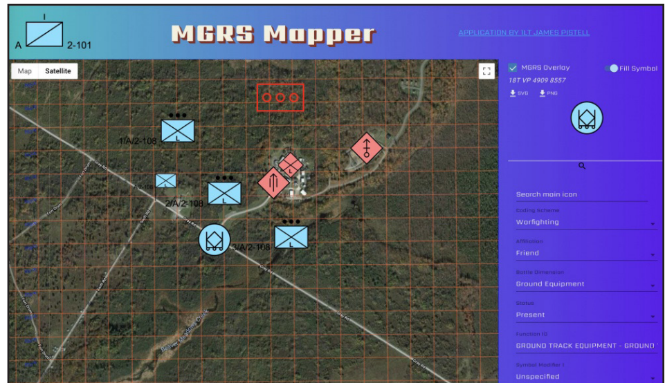
The MGRS-Mapper computer application developed by New York Army National Guard 1st Lt. James Pistell allows users to overlay the military grid reference system on a Google maps image and then create and place tactical and warfighting graphics and symbols on it to be used as an overlay and shared via e-mail. Photo Courtesy.
