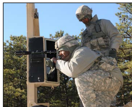
Spc. Jessy Bitwa and Spc. Deshawn Thomas (kneeling) use the bore-sight telescope that is mounted on the AN/TPQ-36 antenna to accurately detect and locate weapons, to align the antenna. The far stake is emplaced at a minimum distance of 100 meters (more than 250 meters preferred) in front of the radar antenna.
