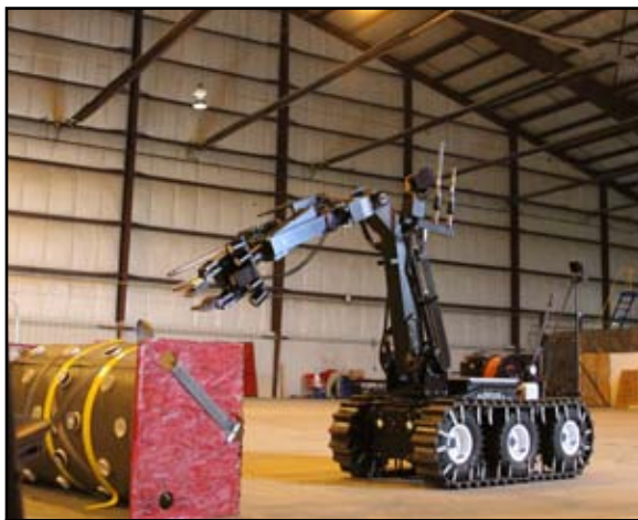
A bomb-disposal robot approaches to heft a 150-pound package during the "robot rodeo" part of the exercise.
