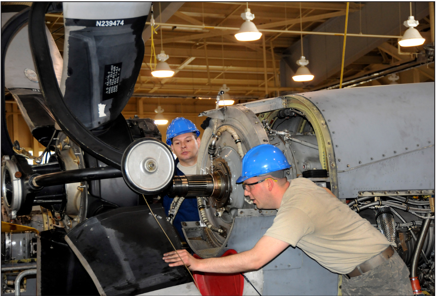
New York Air National Guard Tech. Sgt. Aaron Clause, right, and Tech. Sgt. Dan Weiser guide a prop onto a newly installed C-130 T56 engine. The Air National Guard's 107th Airlift Wing's maintenance team installed the rebuilt engine during sheduled maintenance May 4 to prepare the wing aircraft for deployment to Afghanistan.
