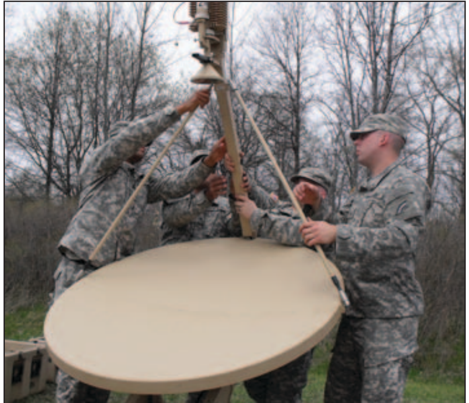
Soldiers from the 42nd Infantry Division TAC 1 assemble a Hawkeye II Satellite System.
