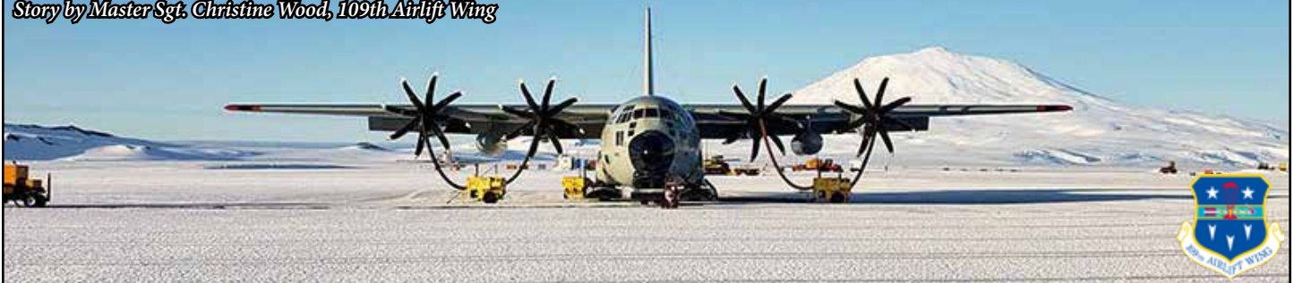
Above, an LC-130 "Skibird" assigned to the 109th Airlift Wing sits at on the skiway at Williams Field, Antarctica, on Feb. 6, 2020. Below, a penguin observes operations at the field. The Wing flies ski-equipped aircraft for Antarctic research. Photo above by Lt. Joshua Bowers and below by Tech. Sgt. Gabriel Enders, 109th Airlift Wing.
