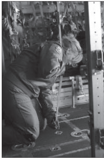
An flight nurse secures a litter system, which converts the C-130 Hercules into a "flying hospital".
