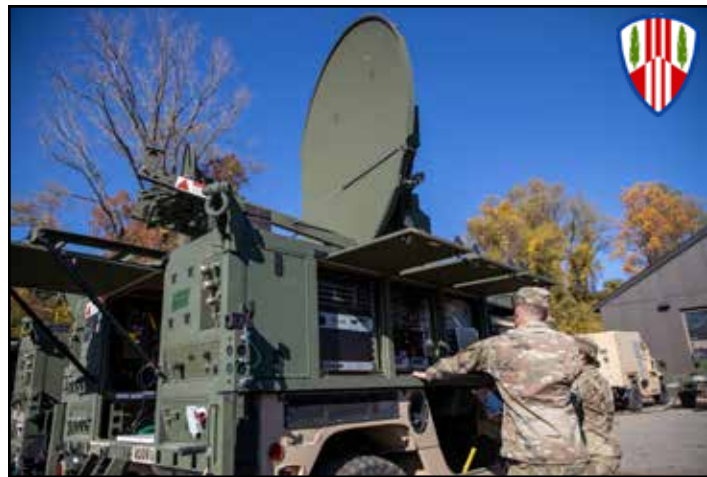
New York Army National Guard Soldiers assigned to the 101st Signal Expeditionary Battalion train on the AN/TSC-156 Phoenix Tactical SHF Satellite Terminal during pre-mobilization training at Camp Smith Training Site in Cortlandt Manor, New York, Oct. 3, 2022.
